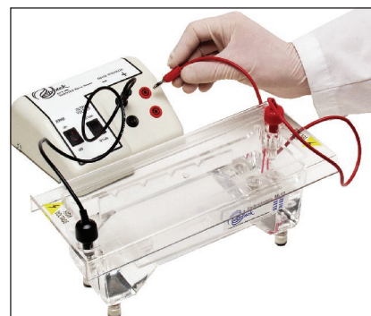
Figure 7.11 Attach the safety cover, connect the power source, and run the electrophoresis.
