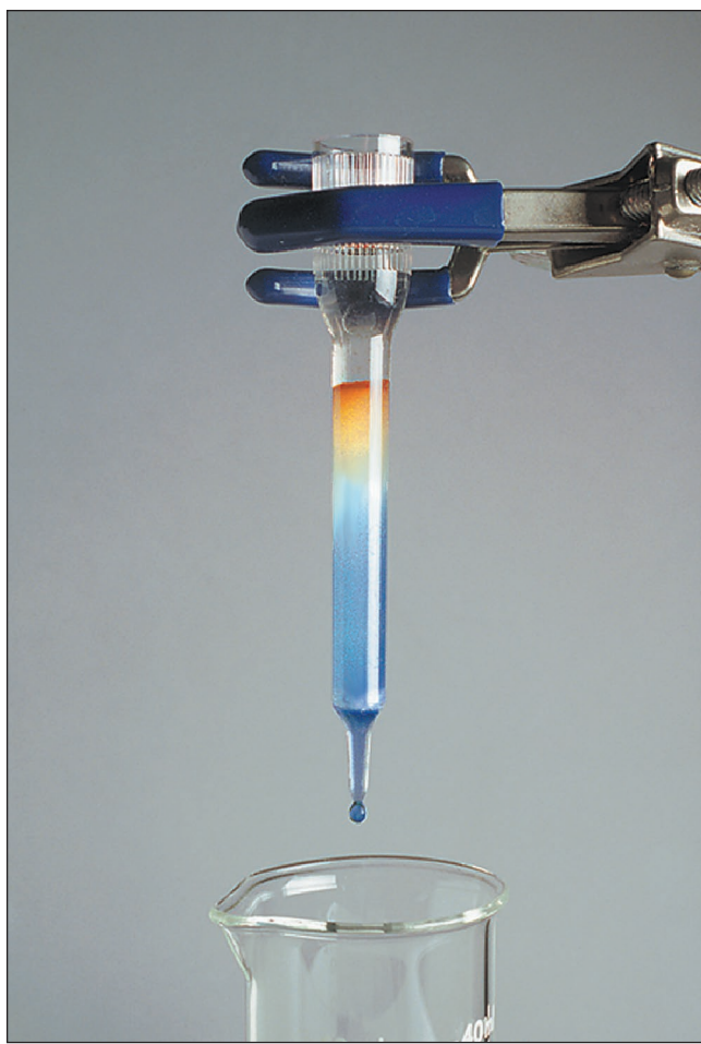
Figure 7.2 Apparatus for column chromatography. A fraction is being collected, drop by drop, in the beaker. Smaller fractions would be collected in test tubes.
