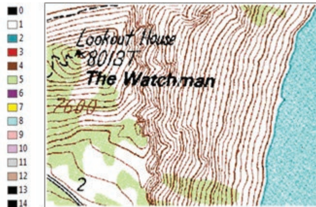
Fig. 2.18. An indexed-color raster stores a colormap that assigns a color to each value in the raster. Source: USGS
