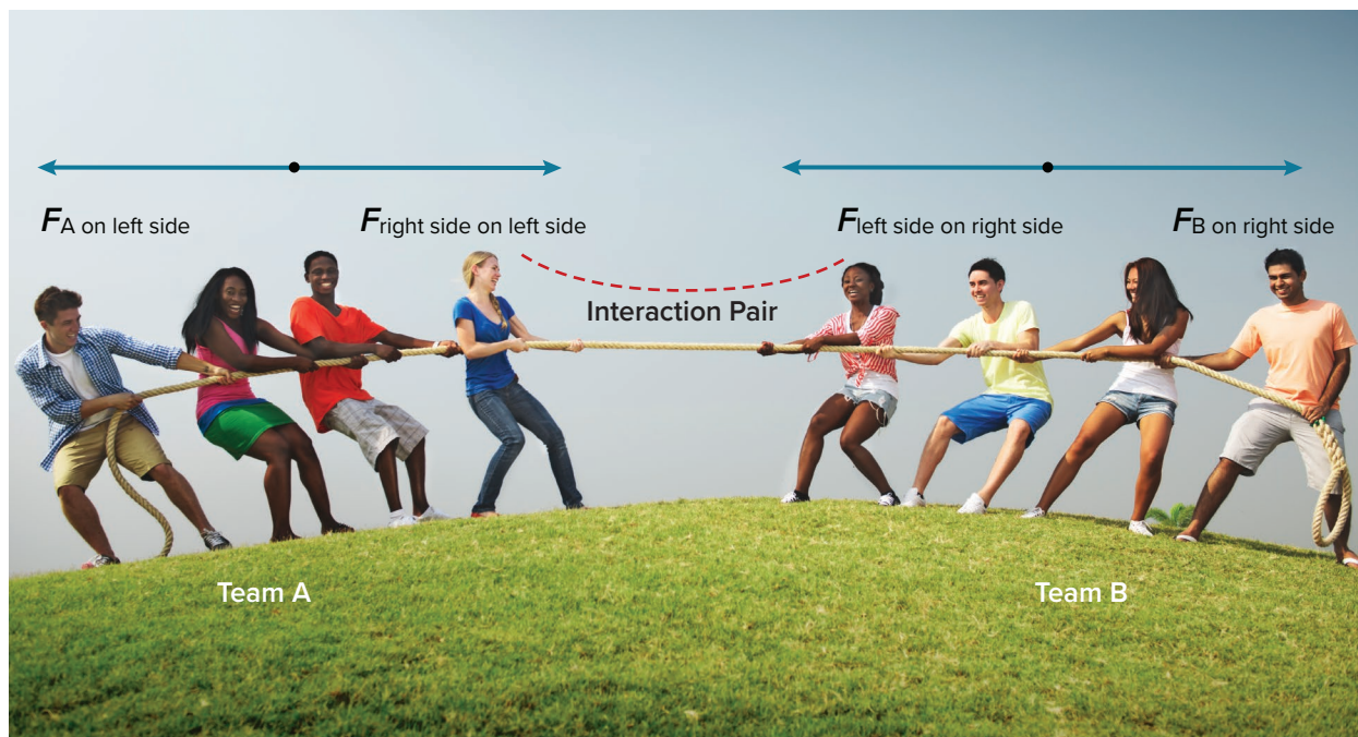
Figure 18 The rope is not accelerating, so the tension in the rope equals the force with which each team pulls.
