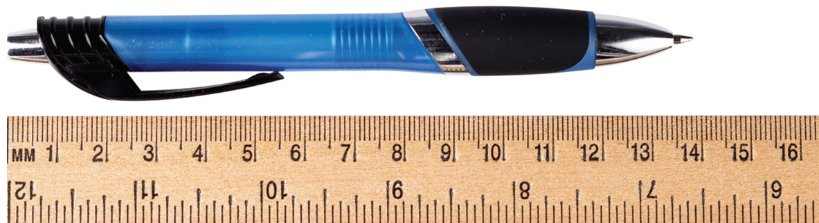
Figure 8 You recorded the length of this pen as 138.1 \text{ mm} .
