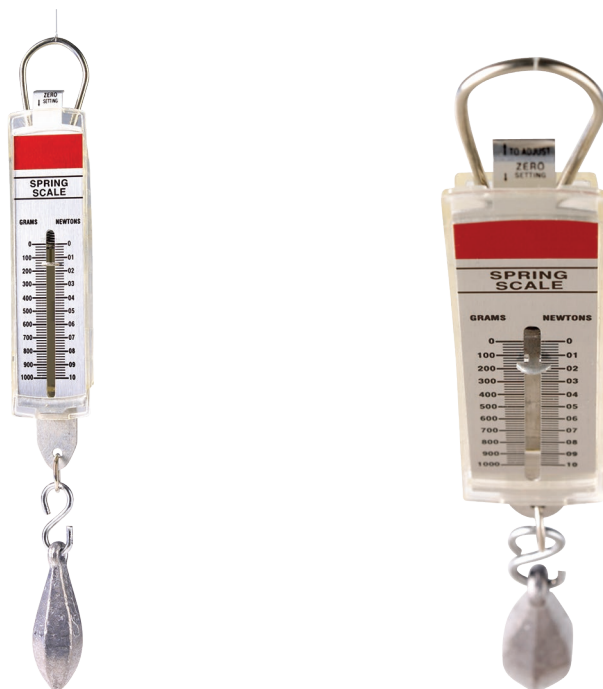
Figure 13 By positioning the scale head-on (left), your results will be more accurate than if you read your measurements at an angle (right).
